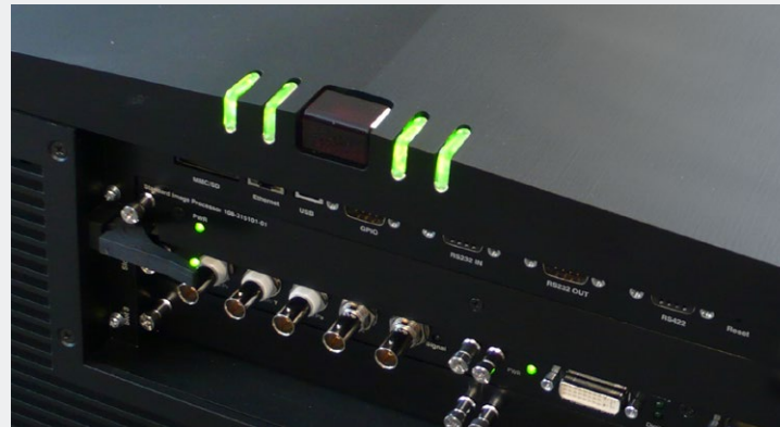
Analog Input, Dual Link DVI input, Video Decoder input, Dual SD/HD SDI input and 3D-ready twin HDMI 1.4 input
