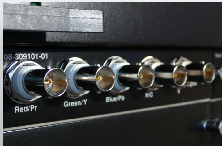
Analog Input, Dual Link DVI input, Video Decoder input, Dual SD/HD SDI input and 3D-ready twin HDMI 1.4 input
